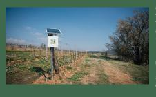
CRNS is based on the detection of neutrons, particles naturally flowing from space and strongly interacting with water molecules. The rate of neutron counts by a detector placed above ground is correlated to the water content in the soil within a volume spanning up to a dozen hectares extension and up to 50 cm depth.
